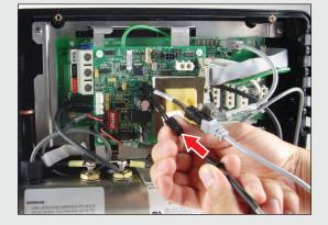
Insert your Control Panel into the second end of the Y-Cable Panel Jack.
