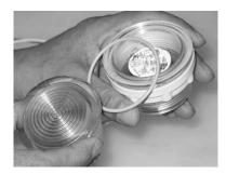
2. Remove lens. Pull bulb straight Out. Verify the o-ring is not damaged and is properly in place.
