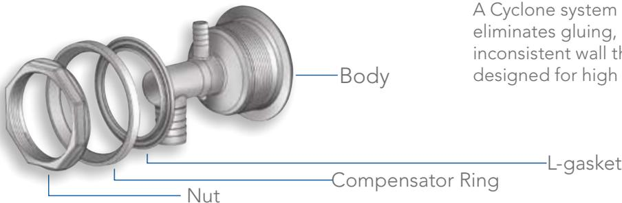
A Cyclone system with compensator ring, nut and L-gasket eliminates gluing, and provides a better seal when facing inconsistent wall thicknesses. A thick flange and body are designed for high resistance to deformation.
