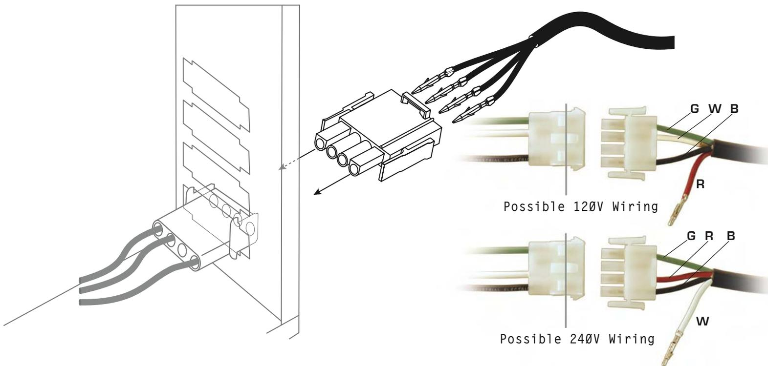
Verify Ozone output connector wiring by using a voltmeter.
