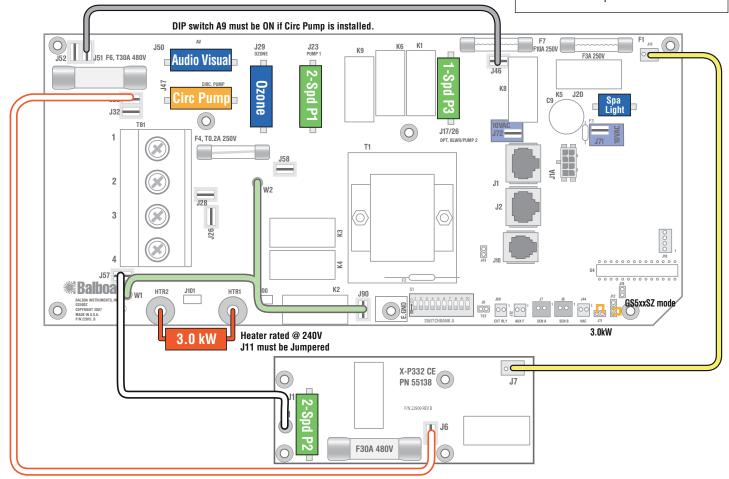
WARNING: Main Power to system should be turned OFF BEFORE adjusting DIP switches.
